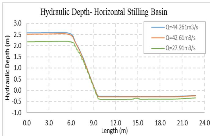
Figure 5. Longitudinal profile- Horizontal basin.
