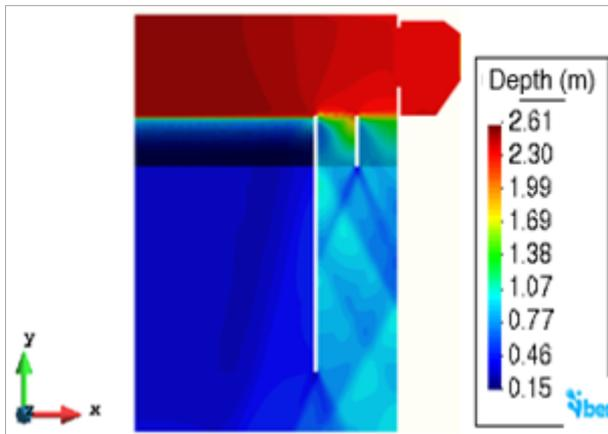
**Figure 3.** Hydraulic depth plan view - Horizontal stilling basin.
