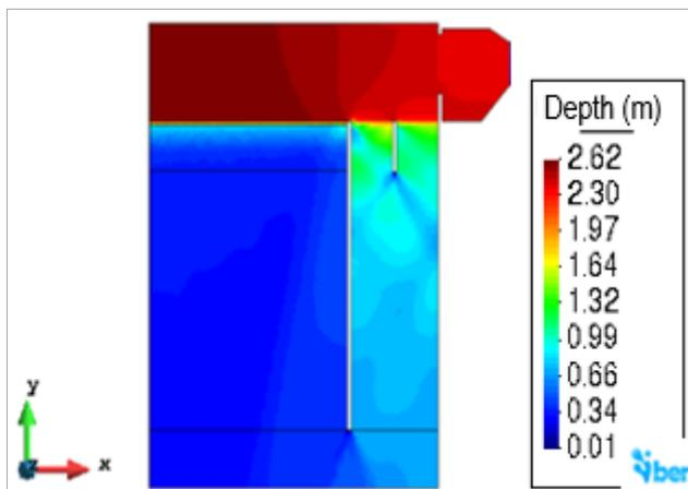
**Figure 4.** Hydraulic depth plan view - 6.08% stilling basin.
