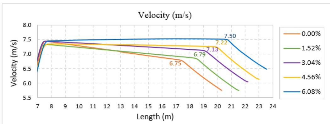
**Figure 11.** Velocity for 5 different slopes.
