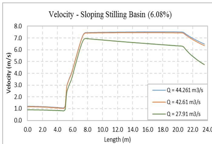
**Figure 8.** Velocity values in stilling basin with slope of 6.08%.
