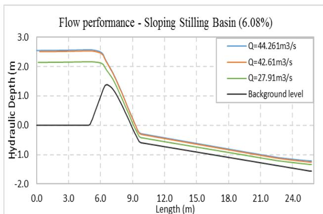
Figure 6. Longitudinal profile- 6.08% slope basin.
