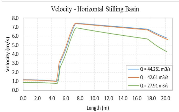
**Figure 7.** Velocity values in horizontal stilling basin.
